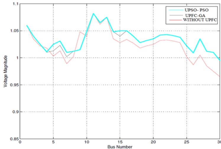
**Figure 4: Voltage Profile with and without Placement UPFC**
